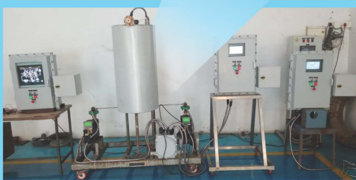
PINCHED TUBE REACTOR
